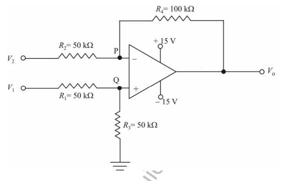
(a) Determine the current flowing through resistance  $R_4$  and the output voltage  $V_0$ . (12)
